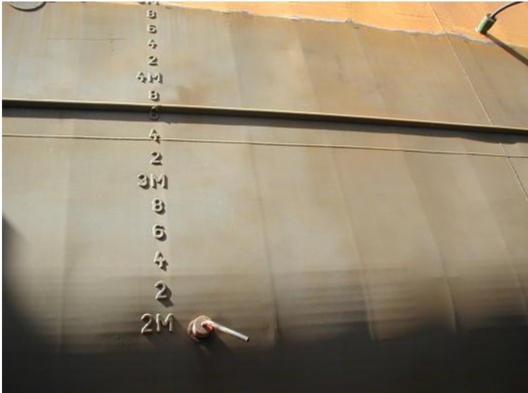
Photo11. LINDA KOSAN underwater part – surface preparation.
