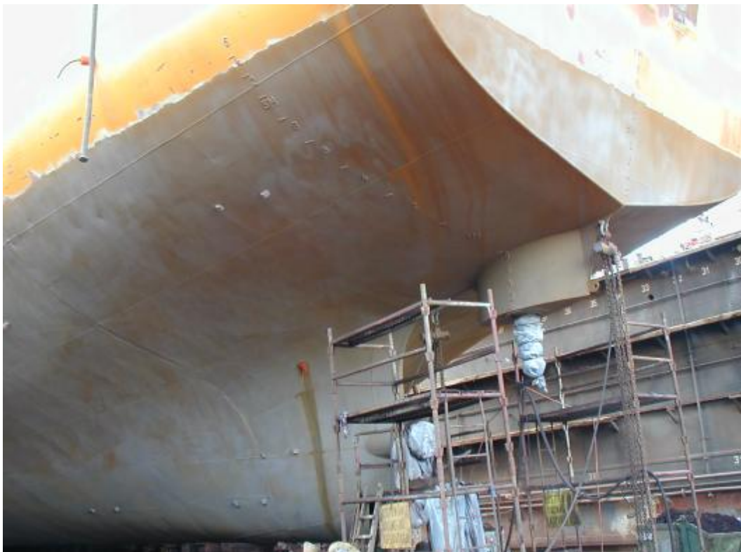
Photo 12. LINDA KOSAN underwater part – surface preparation.
