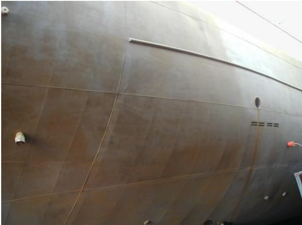
Photo 9. LINDA KOSAN underwater part – surface preparation.
