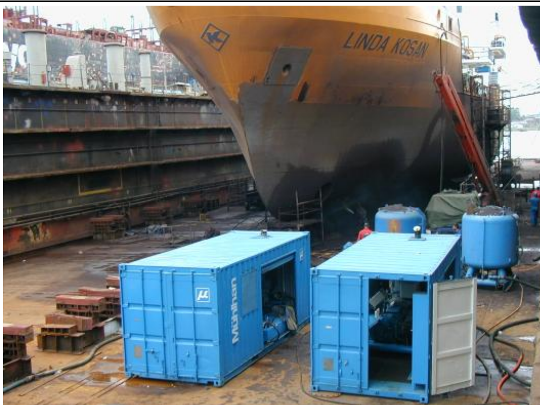
Photo 8. LINDA KOSAN underwater part – surface preparation.
