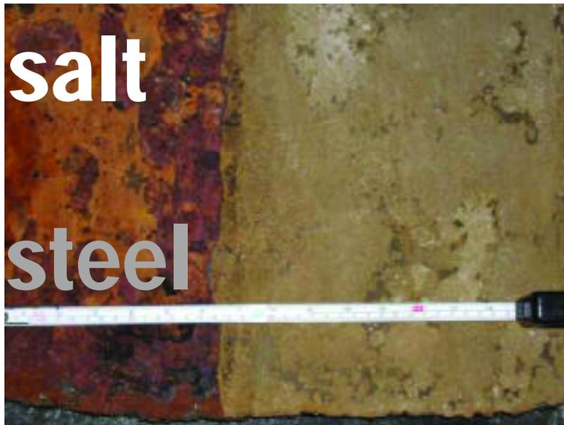
Fig. 1: Heavily corroded steel plate before (left) and after (right) UHP water jetting
