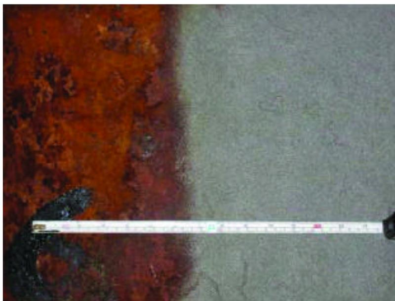
Fig. 2: Heavily corroded steel plate before (left) and after (right) UHPAB water jetting
