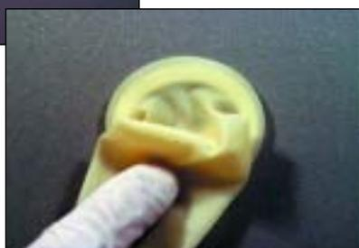
Fig. 4: (right) Adhesive sleeve for soluble salt extraction
