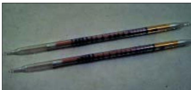
Fig. 5: (above) Ion detection tubes
