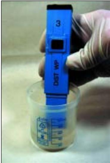
Fig. 7: Pocket conductivity meter
